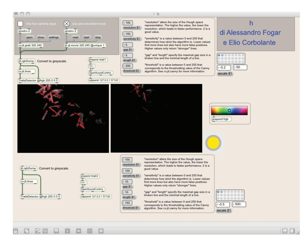
Communication between the computer vision module and the sonification module is via the OSC Protocol<sup>[5]</sup>. This allows easy distribution of the processing load between two computers, one dealing with trace detection and the other with sonification. The two track recognition algorithms send their data separately and are processed by two different sonification modules.
