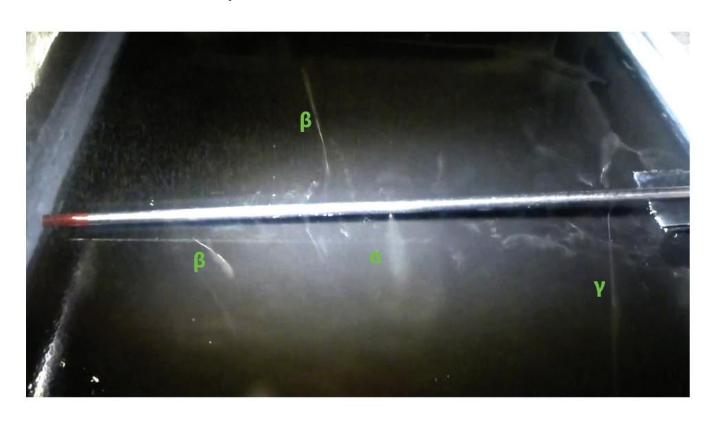
The detection of the traces left by the elementary particles in the cloud chamber is implemented using the *cv.jit* library by Jean Marc Pelletier<sup>[2]</sup>, a collection of objects and tools for computer vision based on Max/Msp/Jitter. The main *external* used for the detection is *cv.jit.lines*. The images are cap-
